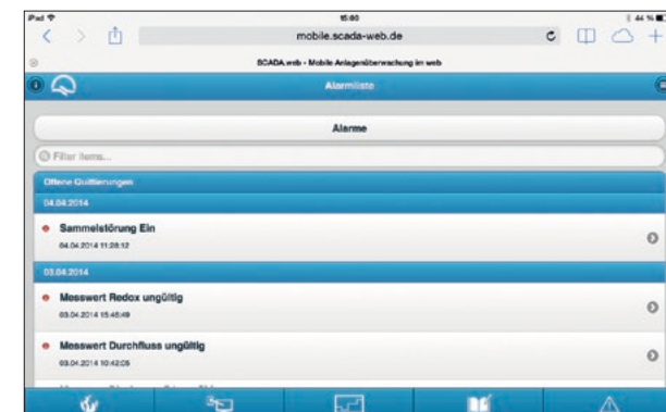
Acknowledging with the SCADA app
